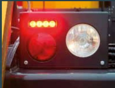
Rear flashing lights supplement the acoustic warning signals for safety inside and outside the vehicle.
