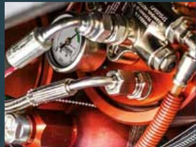
Extinguishing system and diesel particulate filters as per the requirements for tunnelling.
