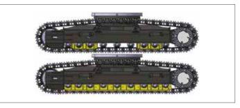
**Track guards:** to provide better protection, track alignment, and performance of machine while travelling. 2 guards per track as standard (double and full-length track guards available as options). These various track guard options provide you with optimal solutions for your extreme applications.
