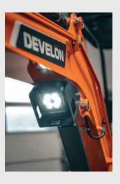
High-illumination LED lamps provide enhanced visibility to the work area to ensure that you can see the work group, particularly the attachment.
